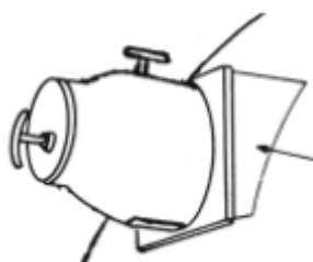
Example of contact protection.
